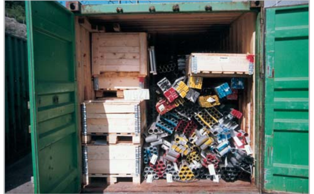
5 off 10m(32.8') span x 24m(78.7') long THAB shelters can be packed in one 20ft container
