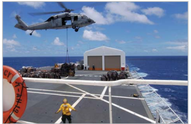
12m(39.4') x 14.6m(48') BVE helicopter hangar on board the ship USNS Mercy
